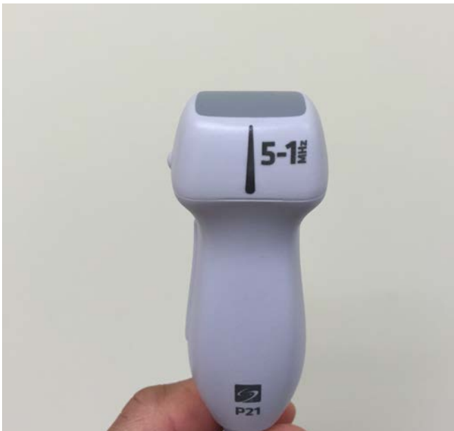
Figure 3 – Phased array cardiac probe.
